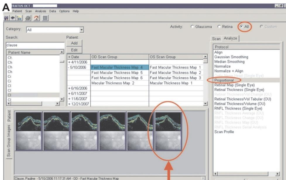
**Fig. 1. A,** Stratus OCT Proportional Process Report 4.0.1 was used to obtain unprocessed images of the vPED for accurate measurements of the vPED heights. **B,** The bottom rectangular-block image shows an undistorted view of the vPED with a total height of 63 mm corresponding to a 2,000- $\mu\text{m}$  scan across the fundus. Thus, the conversion factor for changing the vPED height in mm to  $\mu\text{m}$  is  $31.75 \mu\text{m}/\text{mm}$  (2,000  $\mu\text{m}$  divided by 63 mm).
